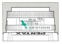
To set the aperture to "A" (Auto), match the green "A" on the aperture ring with the white line index while depressing the aperture A lock button. To off the A position: move the green "A" off the index line while pressing the aperture-A lock button.
