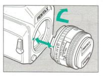
Align the red dot mounting indicators of the camera and lens, and fit and lock the lens on the camera by turning the lens clockwise until it clicks in place.
