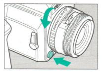
To remove the lens, turn the lens counterclockwise while pressing the lens unlock button.
