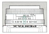
Set the lens aperture to any position other than the A position if using accessories such as a helicoid close-up ring which lacks the lens information contact between the camera and lens.
