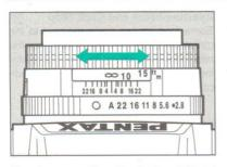
The focus position for taking infrared photographs using an R2 or 02 filter for infrared film differs from that of ordinary visible light photography and requires proper compensation.
